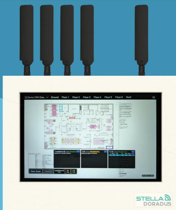
The TestTool is a cellular survey tool, designed specifically for cellular repeater installations. Spectrum mode, Cells mode and the ability to do professional surveys in-building at speed, make this tool an essential piece of test equipment.
