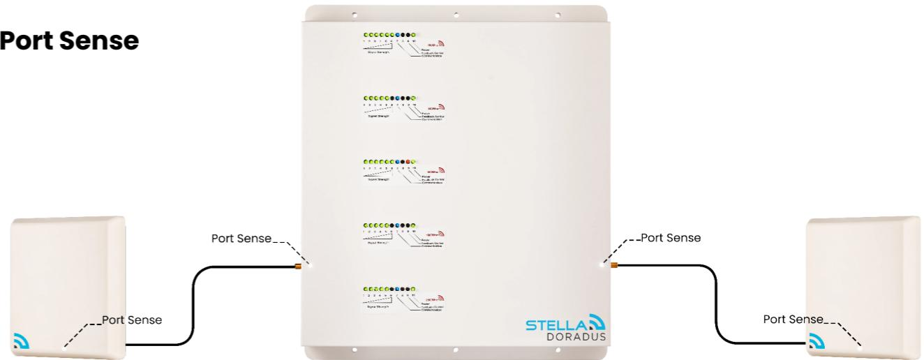
With PortSense, the repeater detects when an antenna is connected to the indoor and outdoor antenna port. Our new smart antennas have an imbedded white LED. There is a corresponding white LED on the port of the repeater. These 2 LEDs will illuminate when the connectors on the cables are terminated correctly and there is a good connection between the repeater and antenna. If the LEDs do not light up, then the cables must be checked.
